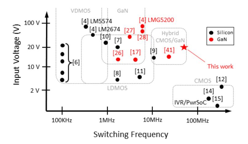
*Input voltage* and *switching frequency* for various converter topologies using silicon and GaN switches
