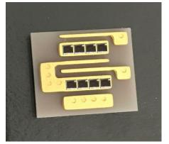
1 cm by 1 cm gold-on-AlN package Excimer laser cutter used for die singulation.
