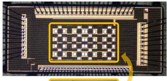
Hybrid GaN-CMOS power converter operating from 40-V power supply.
