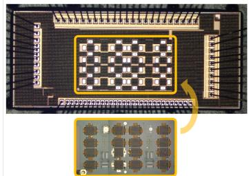
With aggressive die thinning, this can be compatible with C4 bonding.
