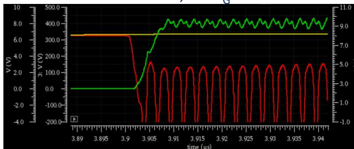
Discrete FET and drive, no R G = out of control
