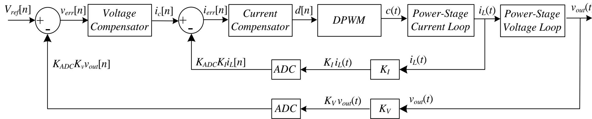
$$v_c[n] = v_c[n-1] + a v_{err}[n] - b v_{err}[n-1]$$
