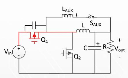
Q1 conducts remainder of interval as in typical buck converter
