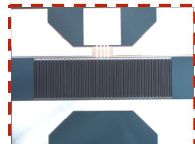
Both W<sub>g</sub>=40 mm and 80 mm devices fabricated
