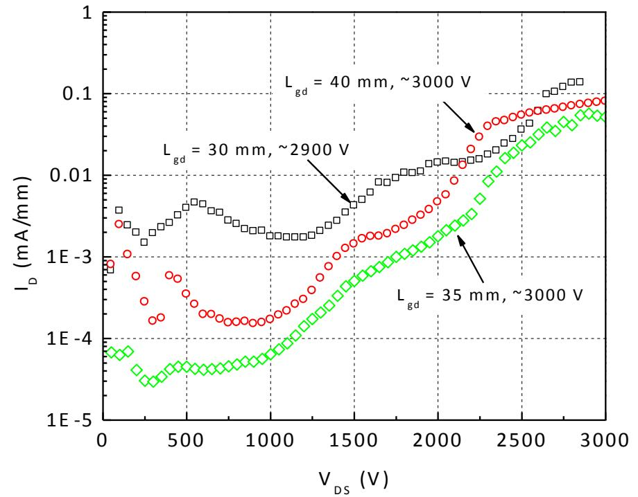
More than 3kV breakdown can be obtained from GaN HEMTs originally designed for 500 V operation
