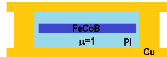
Cross section of a solenoid with FeCoB core
