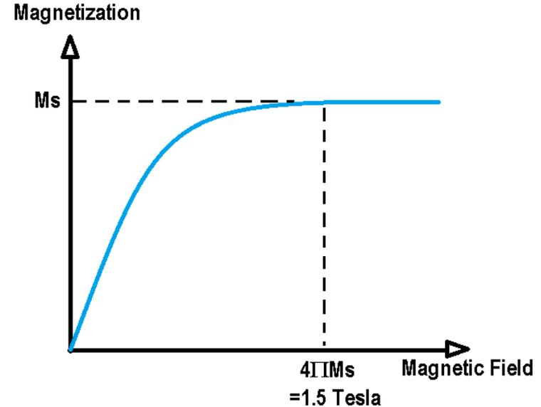
Magnetization Curve of FeCoB along Hard Axis
