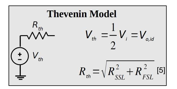
Voltage drop over  $R_{th}$  due to voltage divider formed by  $R_{th}$  and a  $R_L$  . This ratio equals  $\gamma$ .
