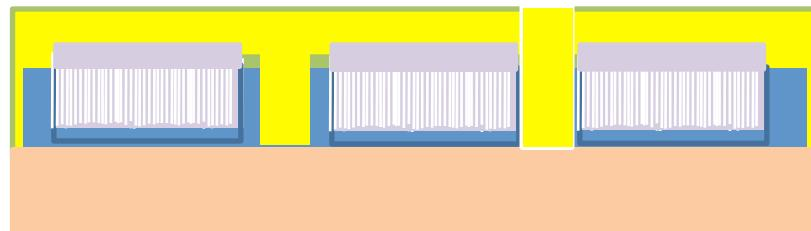
High surface area electrodes on organic substrate with etched foil
