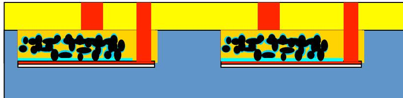
High surface area electrodes on silicon trench;
