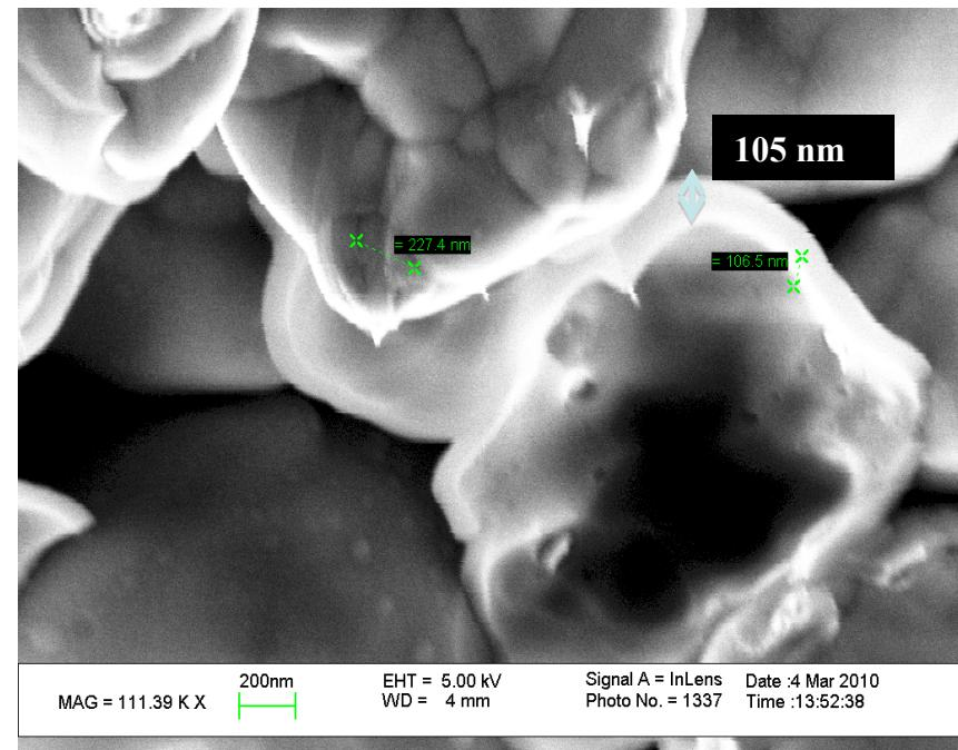
*Cross-section of sintered bottom electrode showing ALD alumina layer*
