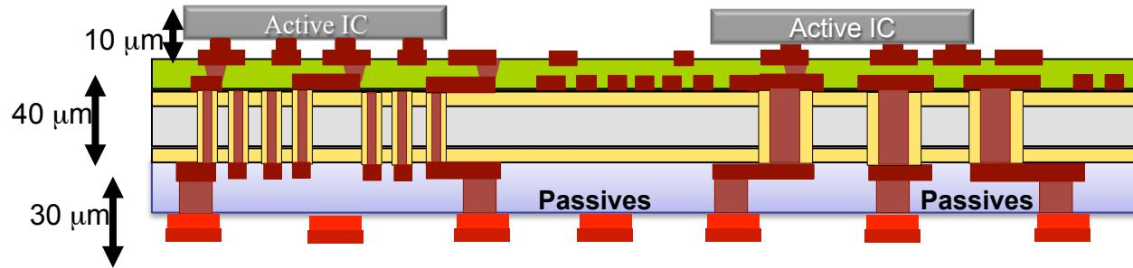
1. Ultra-thin Glass Core  $\sim 30 \mu\text{m}$
