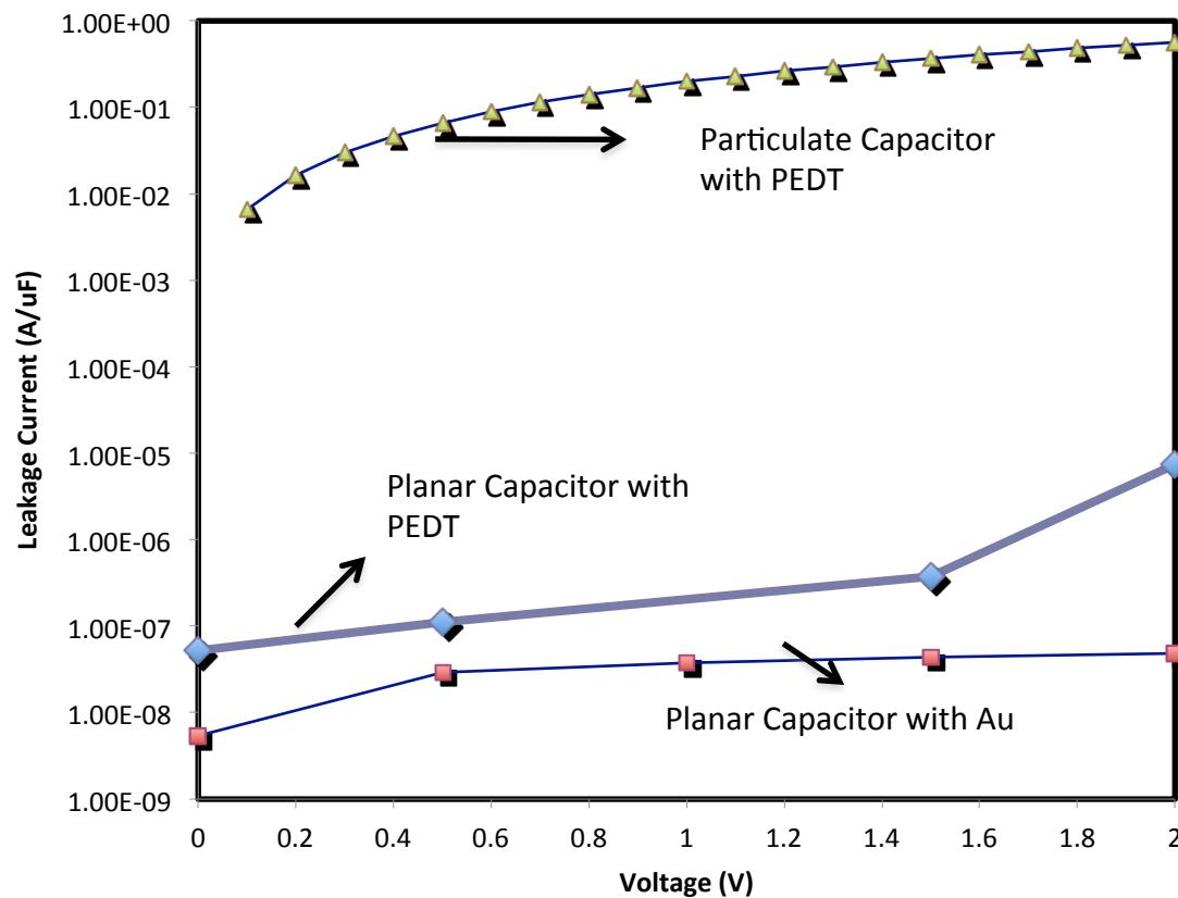
Particulate electrodes using PEDT show very high leakage as compared to planar capacitors.
