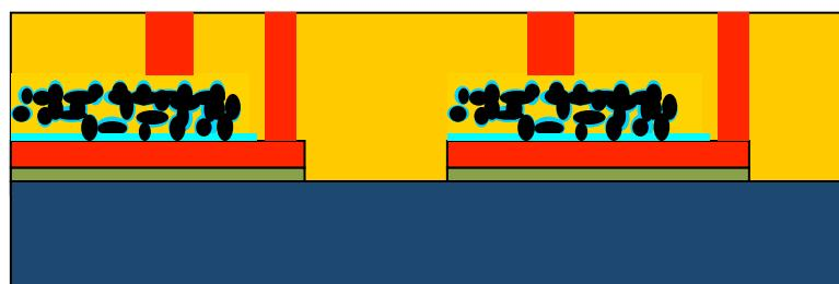
High surface area electrodes on organic substrate with sintered particles
