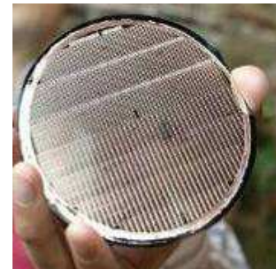
Micro-inductors fabricated on 4 inch Si wafer
