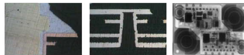
Figure 6:- Cross-sectioning analysis & x-ray image of a DC-DC converter device (based on a printed circuit board substrate).
