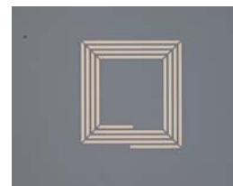
(iii) Aligned : The slits on magnetic film faces to the coil gap.
