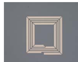
(b) Magnetic film patterning (c) Outlook of the completed inductor
