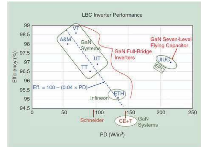
FIG 4 The plot of the inverter FOM shows the UIUC design as an outlier, and traditional designs contain design tradeoffs that are restricted to a particular trend line.
