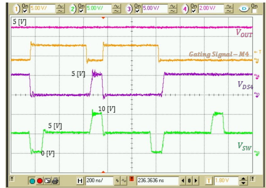
Comparison of the steady state operation of 3-level buck converter for M(D) = 0.5 . a) Conventional controller (left) and b) Skip-duty controller (right). For both waveforms: Ch1. - 5 [V]/div: digital control signal of the low side M4 switch (Fig. 1.), Ch2. - 5[V]/div: V_{SW} , switching node voltage, Ch3. - 5[V]/div: V_{DS4} , Drain-source voltage of the low side M4 switch (Fig. 1.), Ch4. - 2[V]/div: V_{OUT} , output voltage of the converter.
