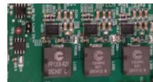
12V POL Multi-phase Buck 85-93% Efficient
