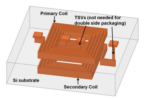
large thicknesses for both coils
