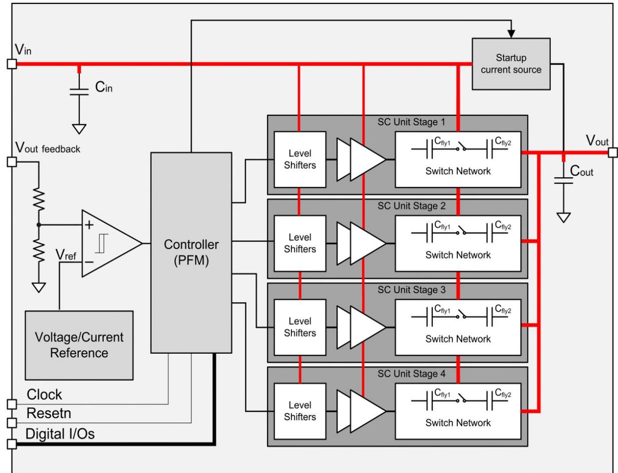
( $V_{in} = 5V$ : Gain=1/3;  $V_{in} = 3.3V$ : Gain=1/2;  $V_{out}=1.3V$ )
