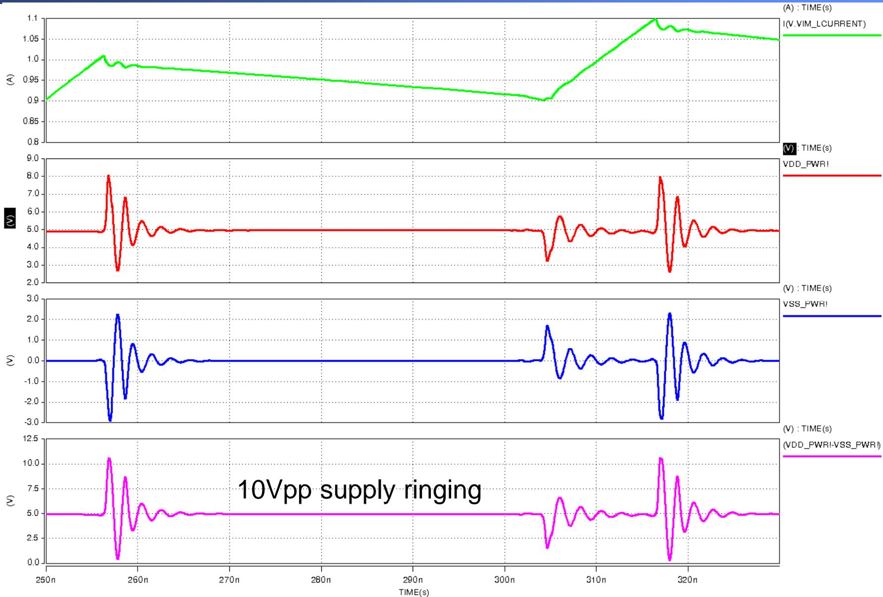
→ Without SiP integration such HF switching is not possible at all due to ringing!
