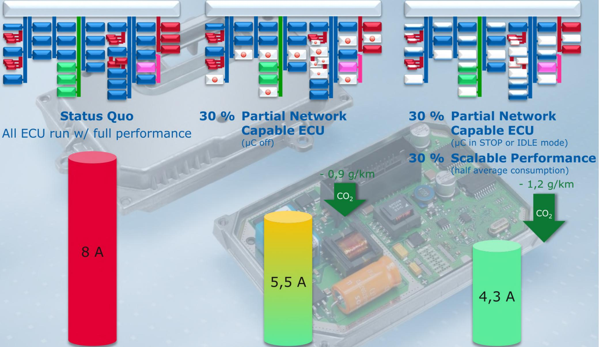
**Assumptions:** Network with 40 ECUs. Average Current Consumption per ECU 200mA. ECUs with scalable performance save 50 % (half average current consumption). Partial Network Mode: Capable ECUs remain 95% of run time in partial network mode with a current consumption of 1mA (μC off) resp. 10mA (μC in STOP or IDLE).
