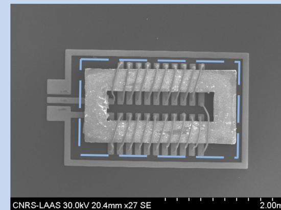
Fig 2: Ferrite-based test inductor with electroplated bottom Cu tracks and gold bond-wire as winding [2].
