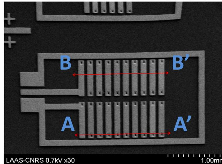
**Fig 3:** Top view of fabricated micro-inductor
