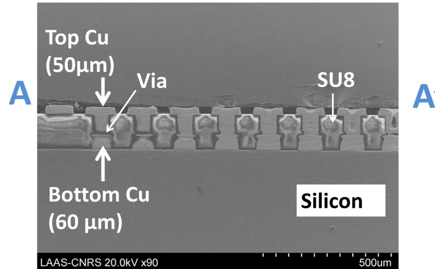
**Fig 4:** Cross section of electroplated top copper tracks-copper vias – bottom copper tracks
