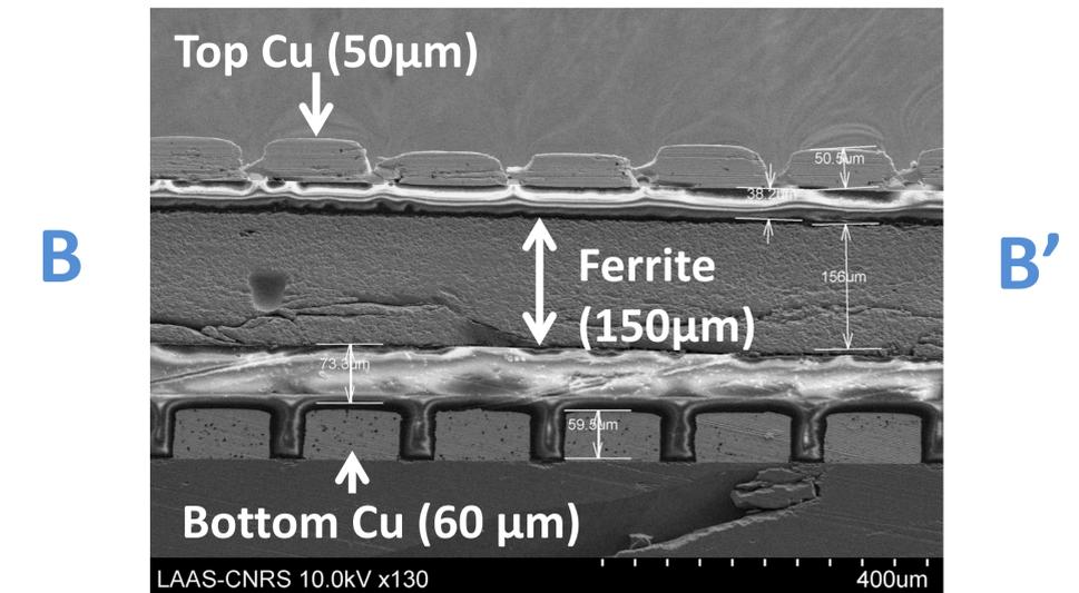
**Fig 5:** Cross section of electroplated top copper tracks-ferrite core – bottom copper tracks (to be added before submission)
