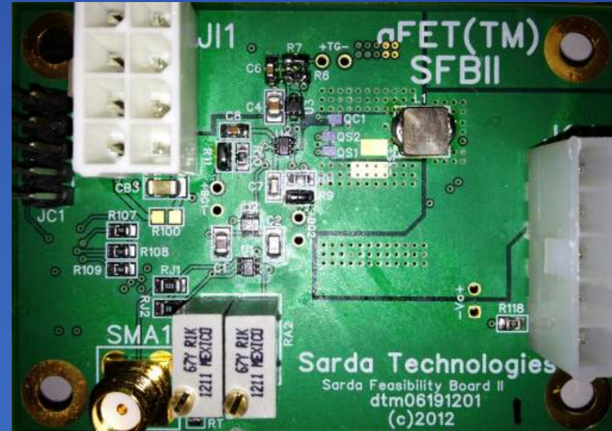
Buck converter circuit using Sarda's GaAs FETs (12Vin, 1Vout, up to 10A)
