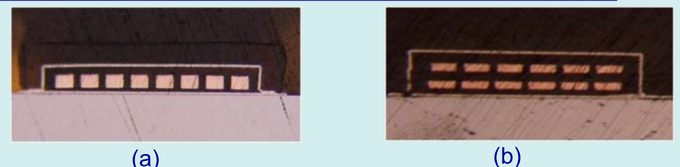
Fig. 5. Cross section of (a) SLM device (b) DLM device
