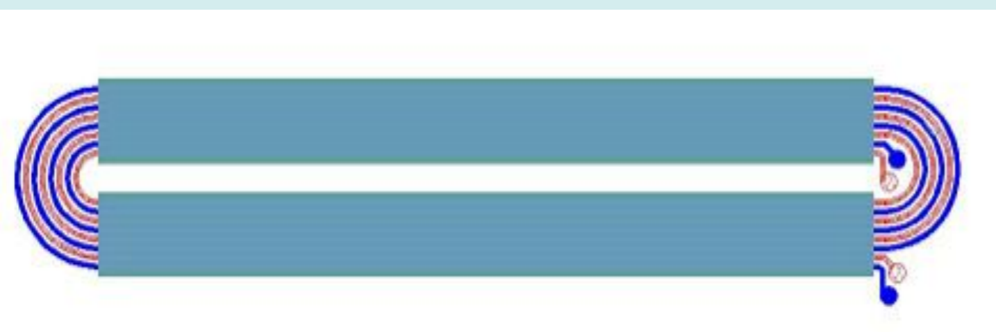
Fig. 1. Top view of a SLM racetrack micro-transformer
