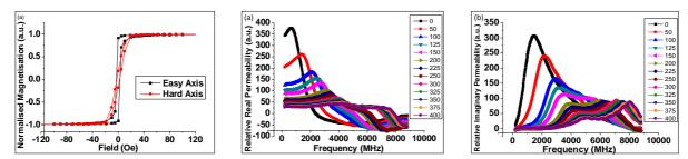
Figure 2: (a) Hysteresis loops in easy and hard axis direction; High Frequency Relative Permeability Spectra of a CoNiFe thin films versus frequency for various bias fields applied (in Oe), (b) real part of the complex permeability, (c) imaginary part of the complex permeability.
