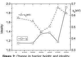
**Figure 2:** Change in barrier height and ideality with rapid thermal anneal temperature, showing improved properties for anneal temperatures around 500°C
