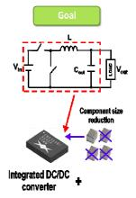
Figure 2: Goal: Reduction of required output capacitors.
