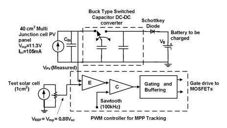
Fig. 1. Block diagram of PV fed SC dc-dc converter based portable battery charger with MPP tracking
