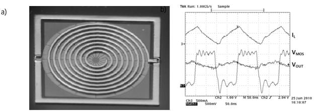
Fig. 1. a) Optical picture of the LC filter (3 mm x 3 mm) with a micro-inductor on top of a 3D capacitor: a magnetic shield (laminated) is integrated. b) Inductor current  $I_L$ , MOS  $V_{MOS}$  and output voltage  $V_{OUT}$  in the buck converter at 5MHz containing the integrated output LC filter.
