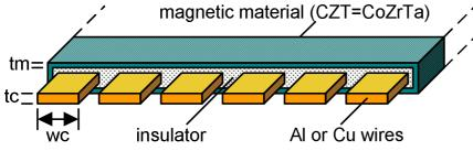
Fig. 1. Inductor structure with magnetic material
