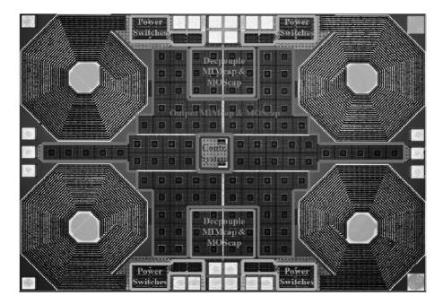
A Fully-Integrated 800mW 4-Phase Step-Down Converter in 130nm CMOS
