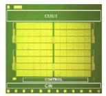
Fig 2. A Fully Integrated Cearbox Capacitive BC DC converter in 90nm CMCS
