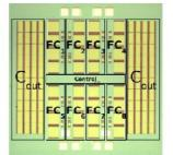
Fig. 1. A 82% Efficiency 0.5% Ripple 16-Phase Folly integrated Capacitive Voltage Doubler in 130nm UMUS
