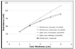
Fig. 2-Plot of inductance versus film thickness for the closed-core inductor.
