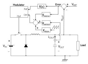
Figure 1: Proposed control: V<sup>2</sup>I<sub>c</sub> control.
