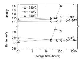
**Figure 1:** Temperature stability of barrier heights and ideality of diodes tested after storage (no bias) .Measurements taken at 25°C.
