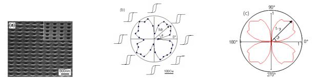
Fig.1 (a) Electrically plated Ni<sub>45</sub>Fe<sub>55</sub> film and imprinted PMMA structure (inset); (b) Angle dependence of normalized remanence; (c) Simulated angle dependence of normalized magnetostatic energy( $\gamma$ ) plotted in inverse polarity.
