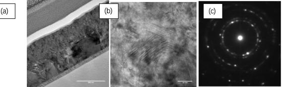
Figure 1: (a) TEM cross section of a CoNiFe electroplated thin film. (b) TEM showing the nanocrystalline structure of the film, (c) SAED showing FCC structure
