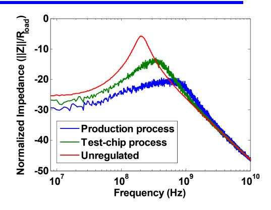
Expect to reach ~50% noise and ~4% power reduction in production process with higher f<sub>t</sub>
